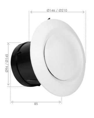
Moulded ABS construction. An inside vent/grille for use with exhaust fans. Ceiling or wall mountable. Adjustable airflow, rotate the center of the unit to open or restrict airflow.
